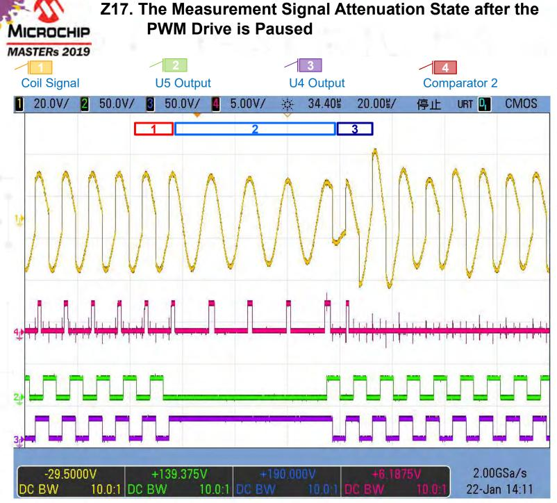
In the process of power transmission, FOD dection requires to suspend the driving of the PWM output to observe the resonant signal attenuation state. This method is quite difficult to implement and the higher the power, the more likely it is to be rushed during the bonding phase. The hardware damage will be caused.
