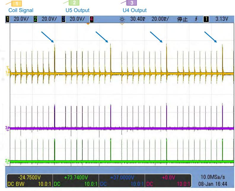
As mentioned above, because the capacitor on the normal working RX is empty, the signal on the abnormal absorption coil maybe judged as having a metalic foreign object. The single driving signal used for detection cannot charge the large capacitor on the RX, so it will not start.
