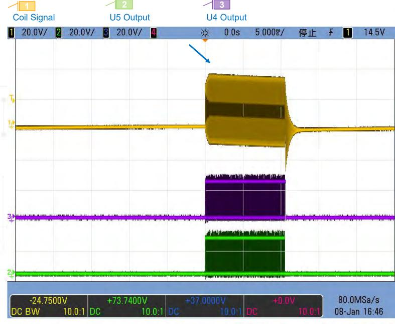
After confirming that there is no metalic foreign object and determing the resonant frequency, it is known that there may be a RX and a drive signal will be sent. If the RX receives this signal, it will start to feed back the data. As long as the data is correct, the power transmission will start.
