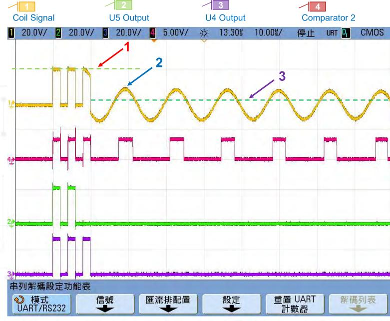
[1]Drive the voltage[2]The first peak afterresonance[3] Set DAC2 discriminationvoltage
