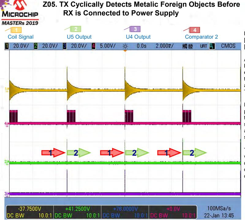
Detection Phases: [1]Short-term driving [2]Measuring procedure
