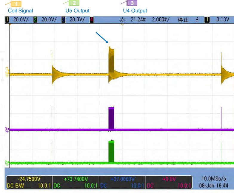
Pre-charge drive is only about 0.5ms which is a very short drive time. Even if there is a metalic foreign object between RX and TX, there will be no heat.
