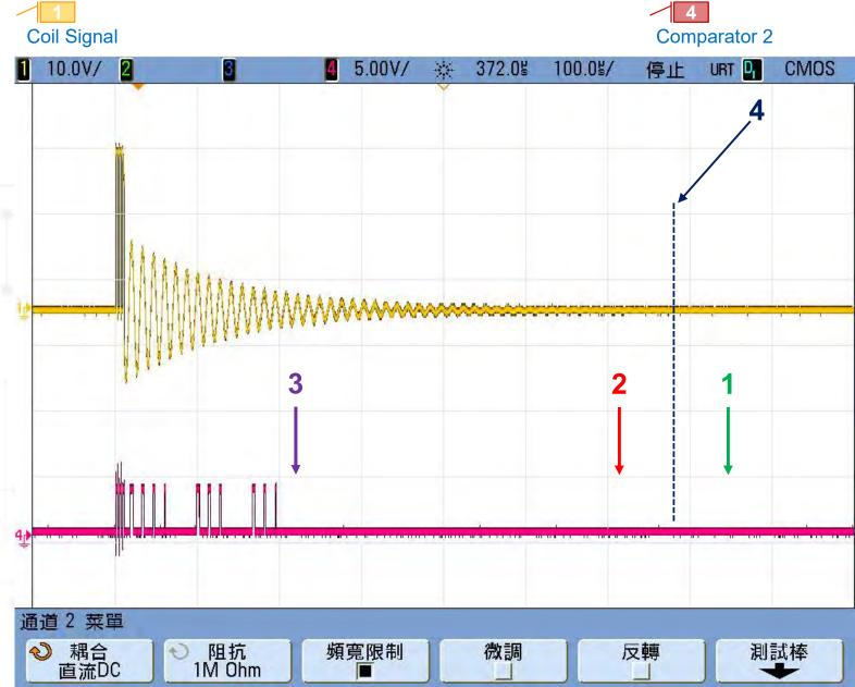
When there is a large metalic object, it will absorb power greatly, so that the attenuation is very fast. At the ending point, the signal will run to the position of [3].
