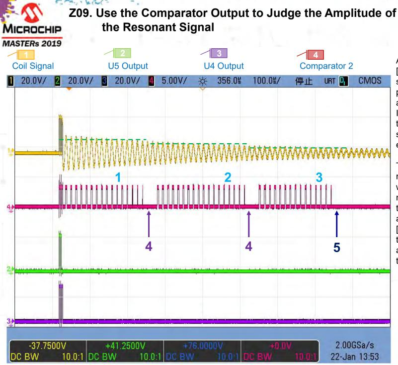
At normal attenuation speed [1] [2] [3] The time of the three segments will be close. The purpose of this design is to avoid moise misjudgment. If the difference between the triggering times of the three segments is too large, it can be excluded as noise.
