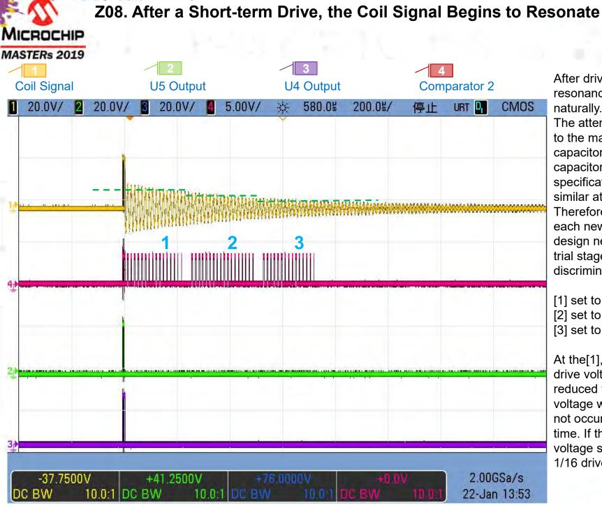
After driving, the coil resonance begins to attenuate naturally. The attenuation rate is related to the match of coil and capacitor. The coil and capacitor of the same specification will have the similar attenuation speed Therefore, the average value of each new coil and circuit of the design needs to be found in the trial stage as the basis for discrimination.
