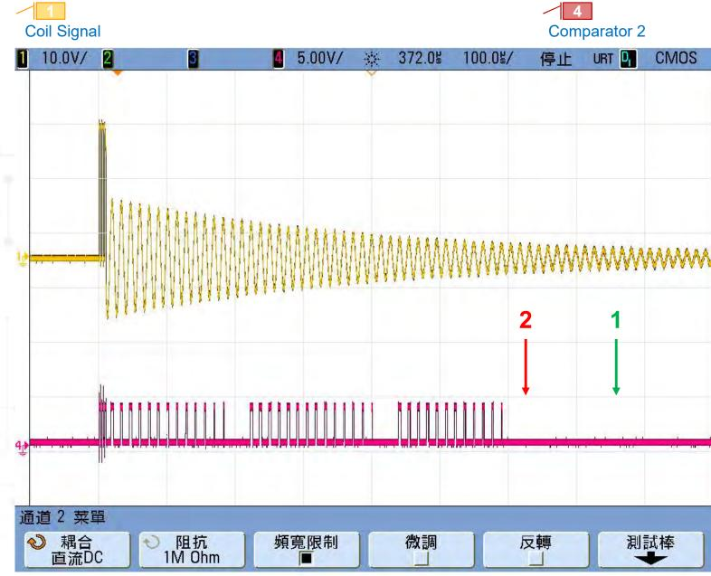
As long as there is a metalic object on the coil, the attenuation of resonance will be accelerated. The end time will reach the position of [2]. This measurement technique is very sensitive. The basis of the judgement is that the electromagnetic power resistance on the coil will absorb the power of the object, which will make the attenuation faster. Therefore, objects that are harmful to wireless charging can be identified.
