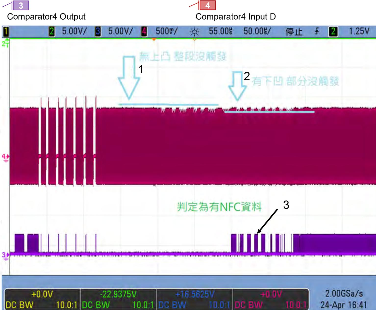
[1] Check the fovea with a higher DAC4 voltage. No trigger indicates that there is no NFC
