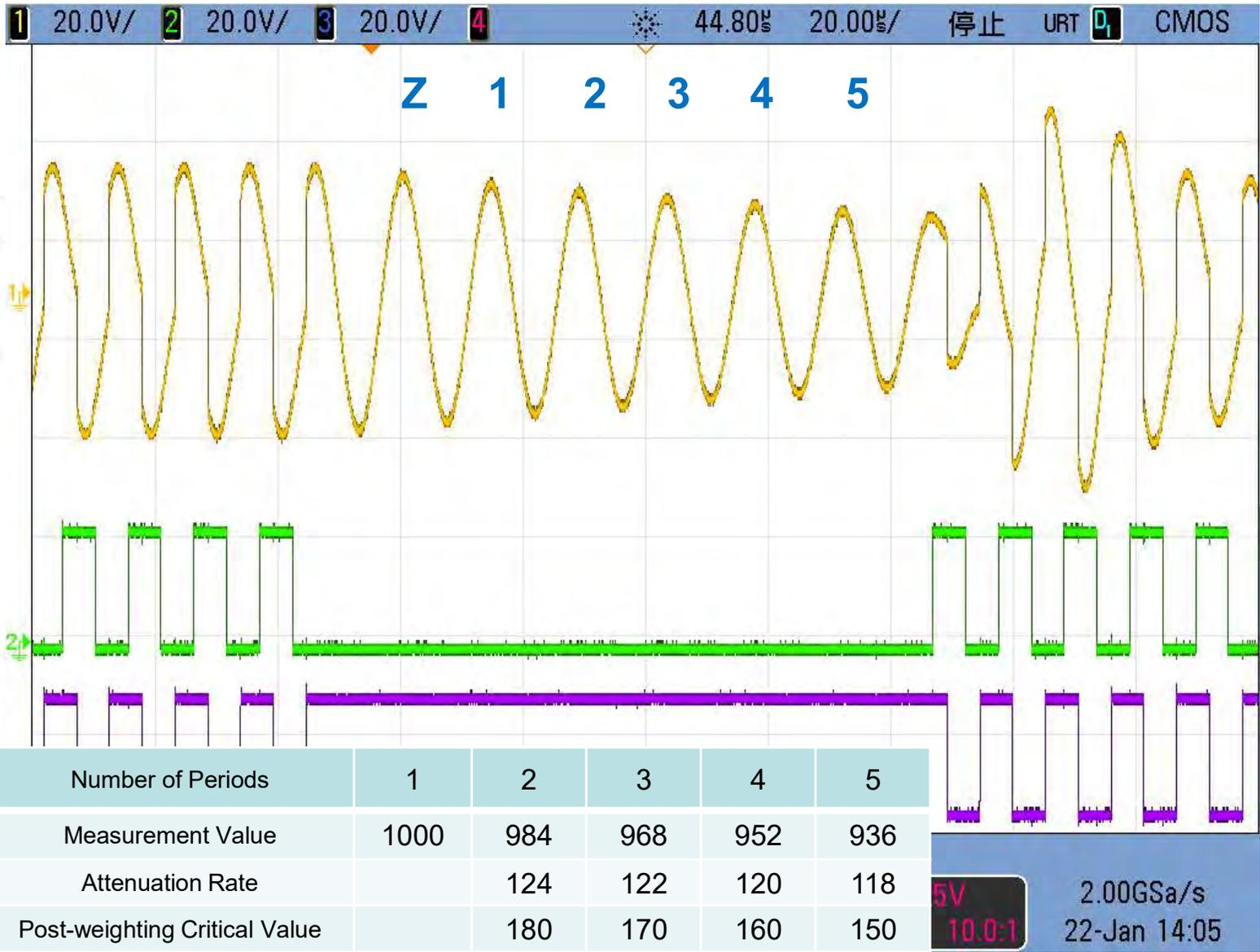
It shows that there are metallic foreign objects. Finally, the calculated slope of [4][5] is 118 which is lower than the critical line 150. It can be judged that there is a metal foreign object, but the power supply will not be cut off immediately. The result of the measurement will be added to the value of the scalar counter. If the value is added to the rated value or more, it is judged that a metal foreign object cuts off the power supply.
