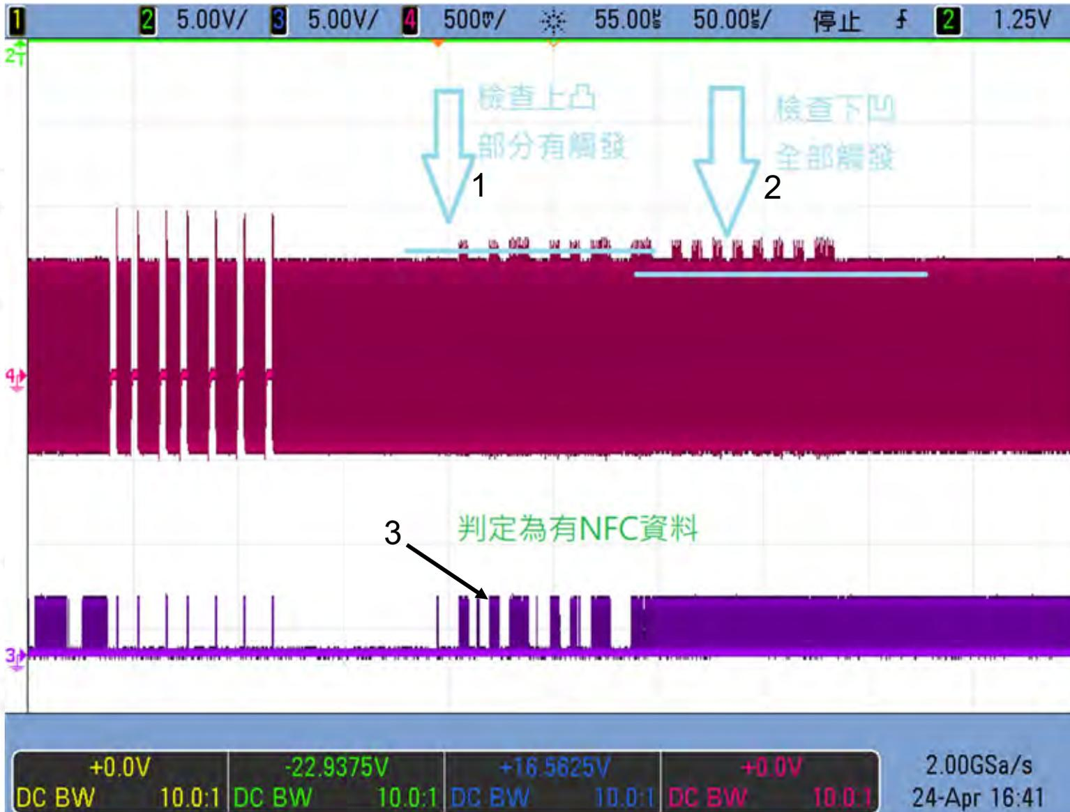
[1] Check the bulge with a higher DAC4 voltage. Some triggers are found to indicate the presence of NFC signal features [3]
