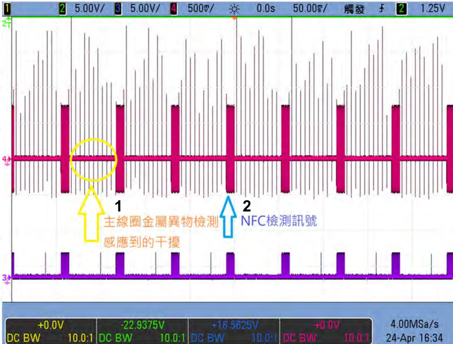
The NFC detection method is to periodically transmit a 13.56 MHz signal on the auxiliary coil.
