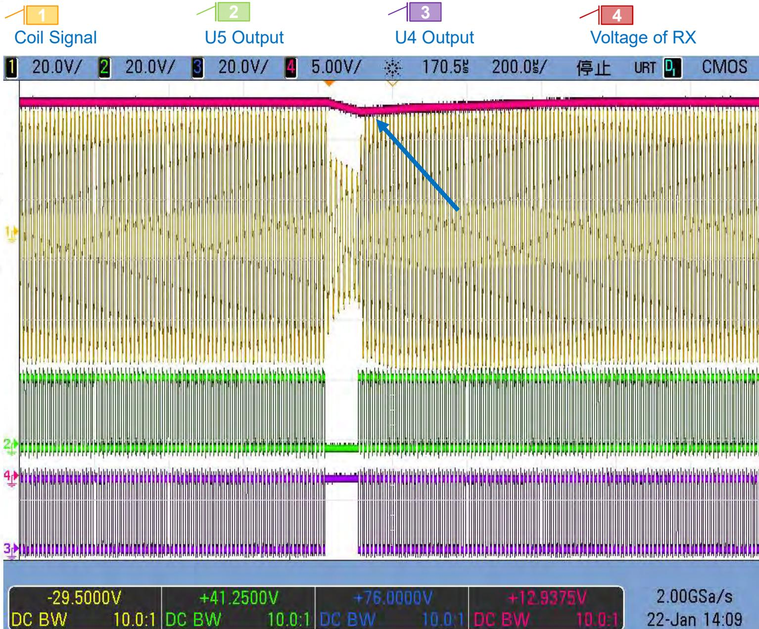
Suspending the PWM drive will stop the power supply from TX to RX. The voltage behind the RX rectifier will also drop. The longer the suspending time is, the greater the voltage drops. The impact of rejoining will also increase. This zone-pause action is not good for the performance of wireless power transmission. High-performance system should reduce the time to interrupt power supply as much as possible.
