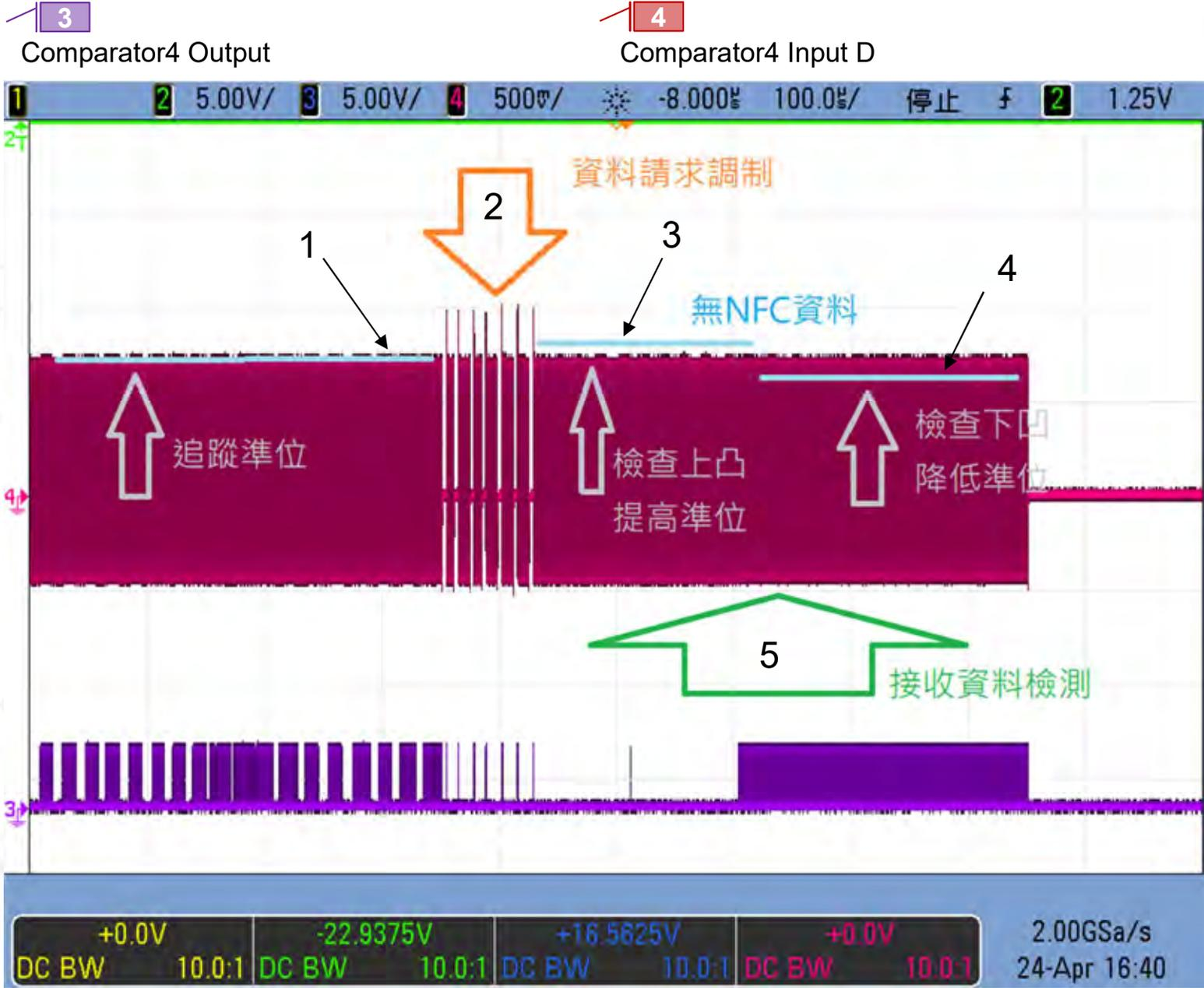
[1] track level section; DAC4 voltage will be close to the peak
