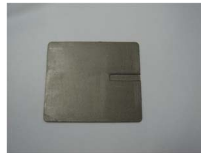
TopFlux Rx Shield & Tx Antenna -Top Rx Shield's Thickness = 0.6mm (TI Rx Shield's Thickness = 0.8mm)
