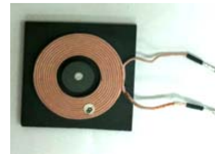
TopFlux Rx Shield & Tx Antenna -Top Rx Shield's Thickness = 0.6mm (TI Rx Shield's Thickness = 0.8mm)
